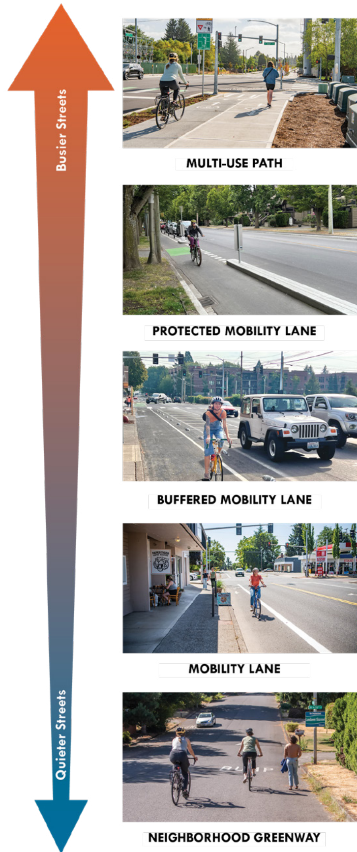
Wider, busier streets need more separation between drivers and BSM users to make them low-stress.
