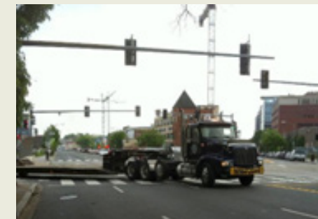
During design, assume trucks will swing into adjacent lanes, which they do in practice. Photo: Nelson\Nygaard
