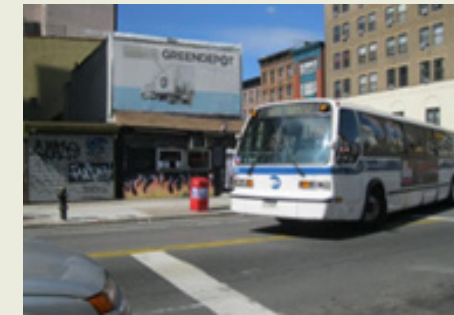
Recessed stop bars allow larger vehicles to make right turns. Photo: Nelson\Nygaard
